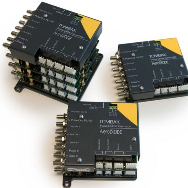
This option allows the user to access multiple output signal while sharing the same power source, the same communication bus and TOMBAK internal signals between stacked boards. For example, output signal from first board can be sent to the second board without any cable thanks to the internal “daisy connector”.
